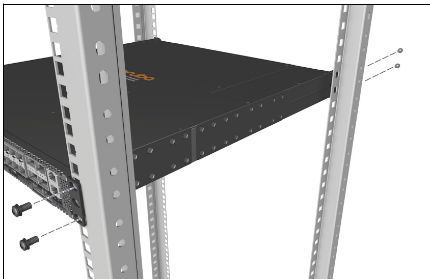
Figure 16: Mounting the switch in a four-post rack
