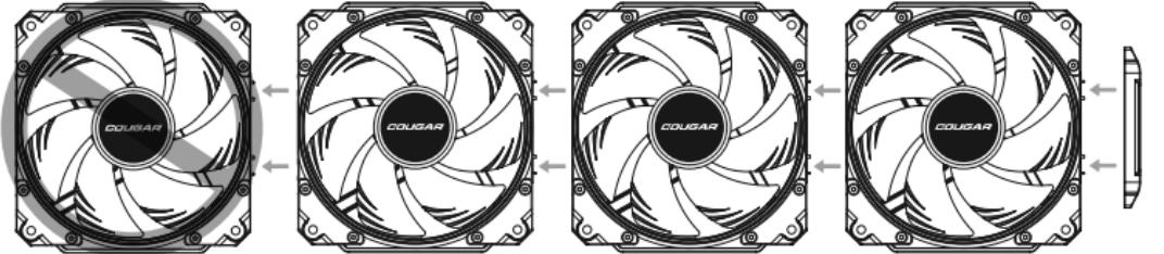
The recommended configuration is no more than three fans due to the limitations of your power source devices. Connecting four or more fans may increase the probability of malfunction due to insufficient voltage.
