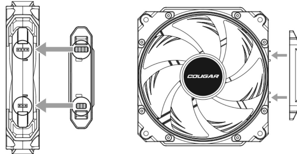
Please align the pins and protruding points of the fan with the connector, and connect them together.
